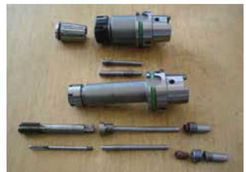
MQL ER-Collet Chuck HSK-A for 2-channel
